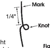
Reinstall cord on top guide of Laserguard. If too tight reposition the knot on cord. Once this operation is complete, you can cut off excess cord.
